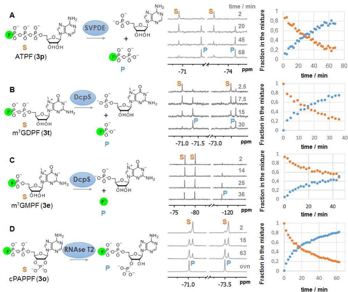
Fig. 4. The use of fluorophosphate nucleotide analogs to monitor the course of enzymatic reactions catalyzed by different enzymes. (A) Hydrolysis of ATPF by SVPDE phosphodiesterase; (B) Hydrolysis of m<sup>7</sup>GTPF by DcpS enzyme; (D) Hydrolysis of cPAPPF by RNase T2 (studies published in H4).
