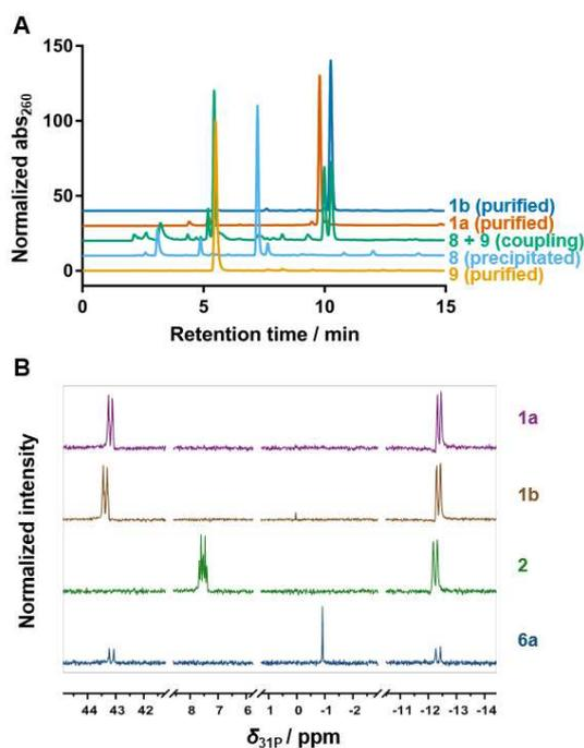
Fig. 14 A) Representative HPLC profiles showing the progress of the synthesis of NAD analog modified with thiophosphate group at the  $\alpha$  position; B) Comparison of  $^{31}\text{P}$  NMR spectra of selected NAD analogs. Data published in paper H10.
